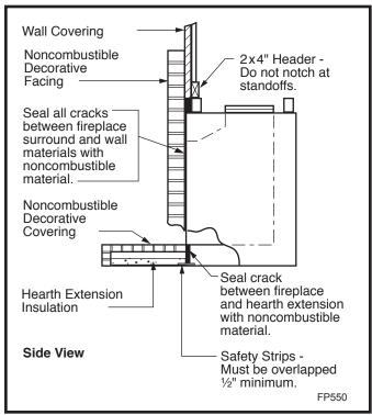
Fig. 26 Sealing gaps.
